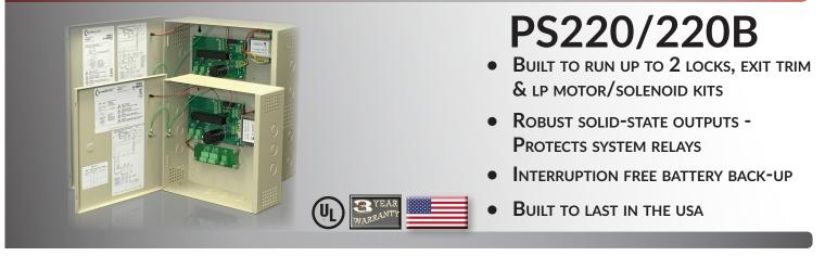
PS220/220B - 110-120VAC input power supplies that deliver (2) amps @ 24VDC to (2) PTC fused outputs. (2) solid-state input triggers, protects system relays from shorts, grounds and surges. It's linear design makes it a perfect match for solenoid & motor driven exit devices, electric locks, electric strikes, and mag locks.
