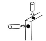
Install Magnet in top or side of the door as shown.
