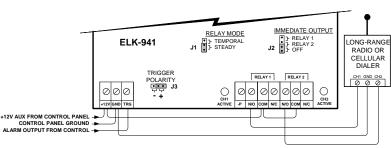
As shown, this hookup is used to activate two channels on a long-range radio or cellular transmitter. Relay 1 activates on steady input; Relay 2 activates on pulsing input. Both relays will stay on until trigger input is removed if both a steady and pulsing input is detected. (Dual mode latch)
