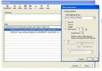
Fade Rate 7 - To turn Off Security Flash or Security Solid the M1 must send Dim Level 18% (Solid) or 19% (Flash) with the fade rate set to "7" to the ID belonging to the Visor Ctrl Receiver. See Table 3b and example below:
