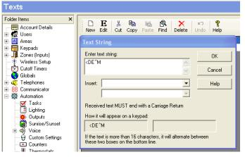
NOTE: Each ID entry after <TS MUST BE TWO (2) DIGITS. e.g 01 to 09, 10, etc. 1 thru 9 will not work.
