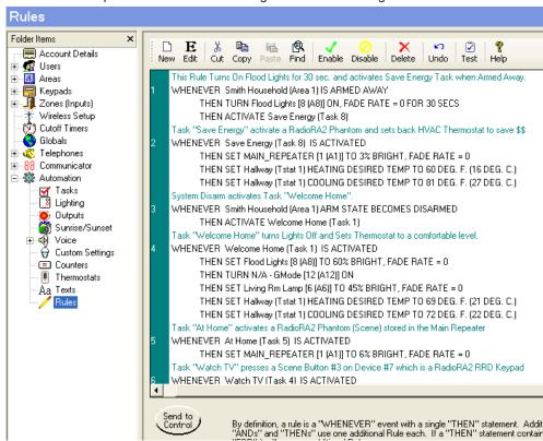
Rule 1 - Turns Flood Lights on for 30 secs. and activates Save Energy Task\* when Armed Away.
