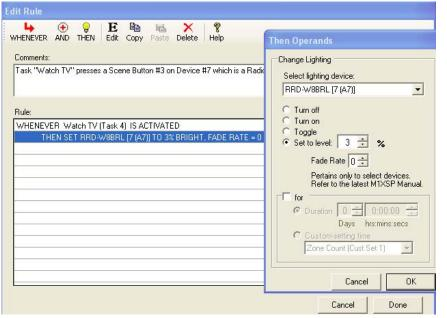
At left is an example of a THEN Operand programmed to press a Keypad Button on Lighting Device 7 (A7) which in this case is a RadioRA2 Keypad [RRD8BRL]. With a Set to Level of "3" and "Fade Rate" of "0" the M1XSLU sends a virtual keypad press command to Button 3 on the selected Keypad device. Other buttons may be pressed (numbers 2 to 20) by changing the Set to Level value. See Table 3b for more info.
