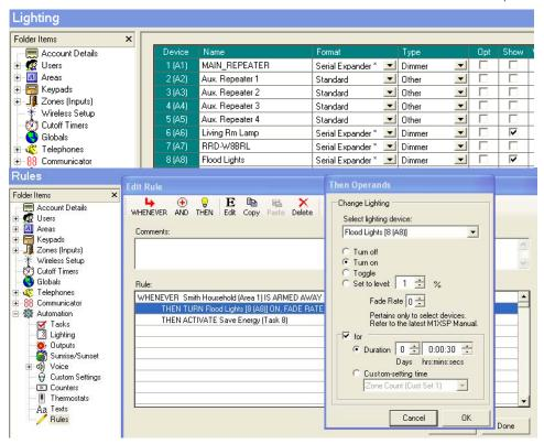
This Rule directly controls 1 light and activates Task=Save Energy when the System is Armed Away.
