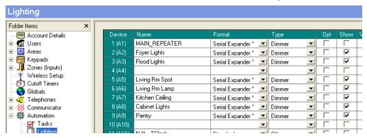
NOTE: Any M1 Lighting Device location that does not have a matching RadioRA2 Device ID to be mapped should be left blank (unprogrammed).
