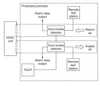
It is typically used to detect smoke in the supply side of the HVAC system but can provide supervision of the return side as well.
