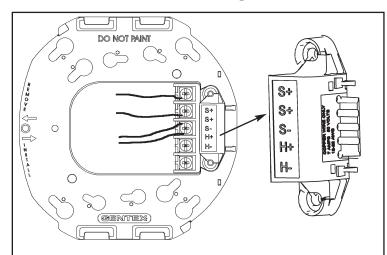
The access holes are provided in the back of the terminal block to allow the voltage to be measured directly without removing the device. Typically this would be done at the end of the line to confirm design criteria. Most measurements will be taken using the S+ and S- locations although access is provided to other locations. NOTICE: Care should be taken to not short the test probes.
