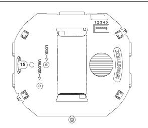
Switch positions 1 and 2 in the down position to select isolated horn and strobe power inputs. Switch 3 selects between temporal or non-temporal tone. Up is temporal. Switch 4 selects between mechanical or high frequency tone. Up is mechanical. Switch 5 selects between high or low dBA. Up is high dBA.
