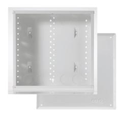
This 14" On-Q enclosure is the perfect solution for a basic structured wiring system. It features larger top openings that make pulling wire easier as well as additional knockouts, more side lances, and side tabs for more flexible mounting. It includes a screw-on cover.
