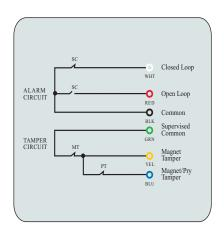
Dual alarm contacts both closed loop, with tamper circuit, closed loop. For built-in EOL resistor configurations and values not shown, contact Potter.
