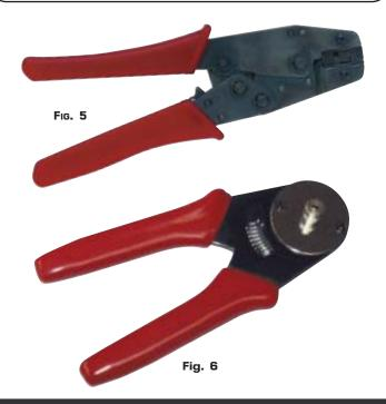
18-22/24-30 AWG WITH TENSION ADJUSTMENT
