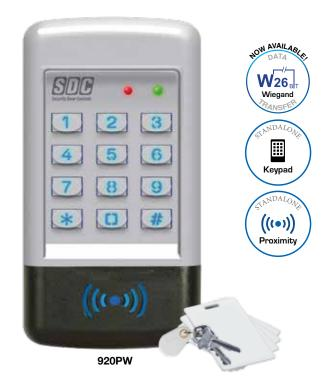
The SDC EntryCheck™ 920 Series indoor/outdoor digital keypads are designed to control access of a single entry point with up to 500 users. Each user is assigned a personal identification number (PIN). Keypad entry of a valid one to six digit code activates one or both of the output relays which releases an electric door lock. Featuring heavy cast vandal resistant housing and cast metal blue backlit keys.
