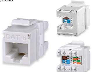
The contact design provides enhanced plug-to-jack connection integrity, protects against damage caused by insertion of 4- or 6-position plugs. Special design features allow these jacks to be terminated with a standard 110 single-position tool or with the Signamax four-pair tool, and are rated for a minimum of 750 plug insertions providing for the highest level of system reliability.
